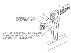
CONTROLTUBEBOLT LOOSEN IN STEP A TIGHTEN IN STEP E
